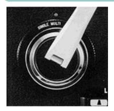
Turn the multiple exposure dial (28) and set the word 'MULTI' to the red dot, then the double exposure prevention is disengaged. The shutter button can be depressed without advancing the film, whenever the shutter is cocked manually.
